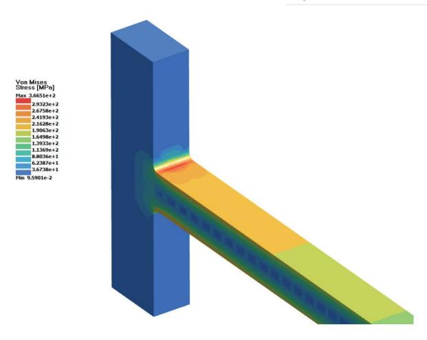
Figure 19: SimSolid - Von Mises Stress
