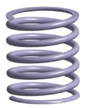
Figure 4: Geometry of the coil spring used in Benchmark 7
