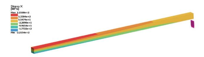
Figure 15: SimSolid – Direction stress acting in a direction parallel to the length of the beam
