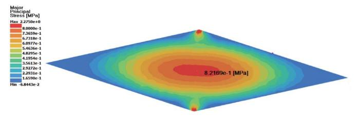
Figure 7: SimSolid - Maximum principal stress on plate lower surface - Benchmark 4
