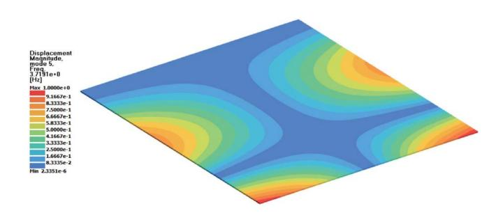
Figure 14: SimSolid - Displaced mode shape - Mode 5 - 3.72Hz - Benchmark 7
