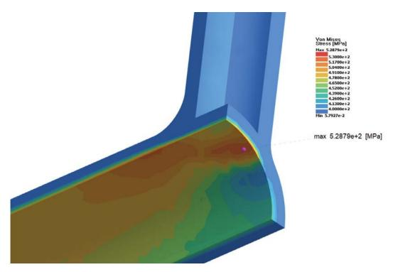
Figure 3: SimSolid - Contours showing Von Mises Stress
