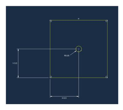
Figure 8: Geometry of the plate with hole benchmark
