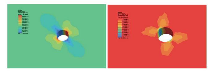
Figure 10: SimSolid maximum principal stress (left) and minimum principal stress (right) – Benchmark 5 – Plate with hole – Maximum accuracy setting
