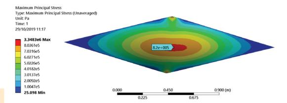
Figure 6: Traditional FEA approach - Maximum principal stress on plate lower surface
