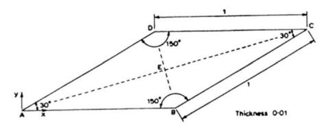
Figure 5: The geometry of the skewed plate
