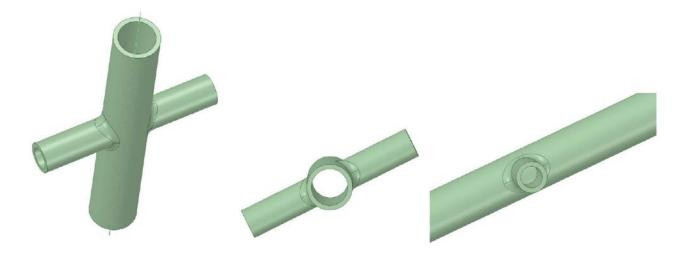
Figure 1: Geometry of the pressurised pipe with intersecting trunnion
